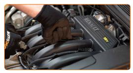
Unscrew the ignition coil bracket. Use a drive socket #10. Use a ratchet wrench.
