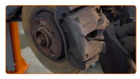
10 Remove the brake caliper.
