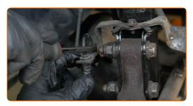
Unscrew the brake hose fastening bracket from the shock strut. Use a drive socket #10. Use a ratchet wrench.
