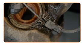
Remove the wheel hub from the steering knuckle. Use a pin punch. Use a hammer.
