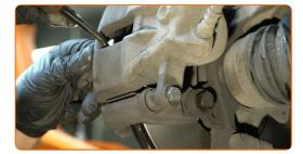
Clean the brake caliper bracket fasteners. Use a wire brush. Use WD-40 spray.
