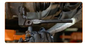
Detach the driveshaft from the steering knuckle.
