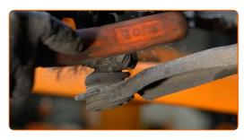
Unscrew the ball joint fastening to the steering knuckle. Use a combination spanner #16. Use a drive socket #16. Use a tap wrench.
