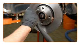
17 Remove the brake disc.
