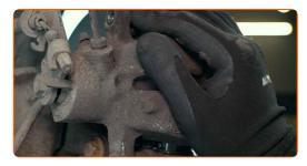
Tighten the brake caliper fasteners. Use a combination spanner #13. Use a drive socket #13. Use a torque wrench. Tighten it to 30 Nm torque.
