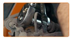
g Remove the brake caliper.
