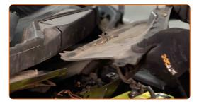
Unscrew the filter housing fastening bolts. Use a Phillips screwdriver.
