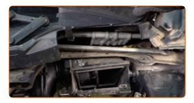
Reinstall the air filter housing.
