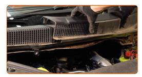
Unscrew fixing bolts of the protective cover. Use a drive socket #10. Use a ratchet wrench.
