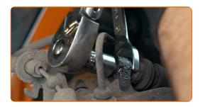
g Remove the brake caliper.
