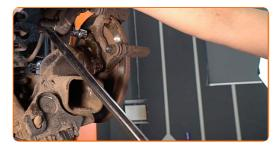
Remove the caliper bracket.
