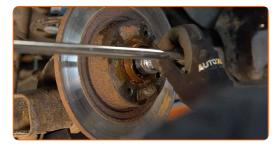
Remove the brake disc assemled with the wheel hub bearing.
