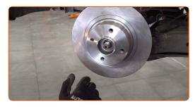
Tighten the hub. Use a drive socket #30. Use a torque wrench. Tighten it to 220 Nm torque.
