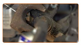
Remove the brake pads. Use a crowbar.
