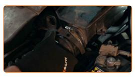
18 Tighten the air duct clamp.
