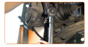
70 Secure the brake hose fastening bracket.
