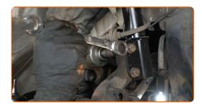
Release the fastener that connects the control arm ball joint to the steering knuckle. Use a flat metal-working chisel. Use a hammer.
