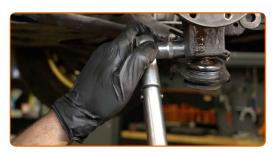
Screw the nut of the drive shaft. Use a drive socket #30. Use a ratchet wrench.
