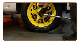
Tighten the wheel bolts using a criss-cross pattern. Use wheel impact socket #17. Use a torque wrench. Tighten it to 105 Nm torque.
