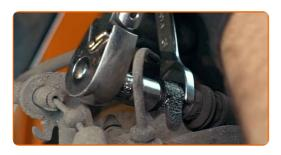
g Remove the brake caliper.
