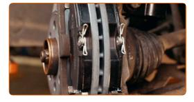
Treat the brake caliper piston. Use a nylon cleaning brush. Use a brake cleaner.
