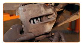
Tighten the brake caliper fasteners. Use a combination spanner #17. Use a drive socket #13. Use a torque wrench. Tighten it to 72 Nm torque.
