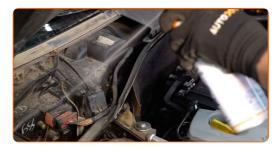
Unscrew the fasteners of the cabin filter housing cover. Use a Phillips screwdriver.
