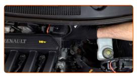
Screw the filter housing fastening bolts. Use Torx T25.
