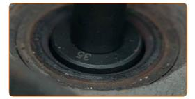
Clean the wheel hub bearing retaining ring. Use a wire brush. Use WD-40 spray.
