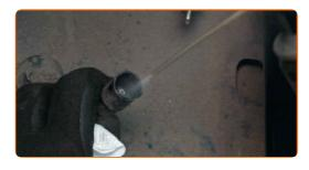
Attach the ABS sensor connector.
