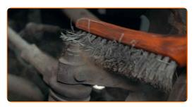
Clean the fasteners connecting the ball joint to the suspension control arm. Use a wire brush. Use WD-40 spray.
