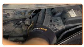
Screw in the fasteners of the cabin filter housing cover. Use a Phillips screwdriver. 12
