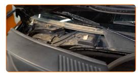
Clean the cabin filter housing and cover. Use all-purpose cleaning spray. 6
