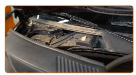
6 Clean the cabin filter housing and cover. Use all-purpose cleaning spray.
