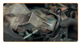
Clean the mounting seat of the engine mount. Use a wire brush. Use WD-40 spray.
