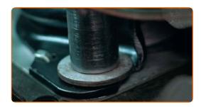
Screw the new engine mount to the bracket. Use a drive socket #16. Use a ratchet wrench.
