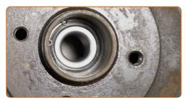
Clean the hub bearing mounting seat. Use all-purpose cleaning spray.
