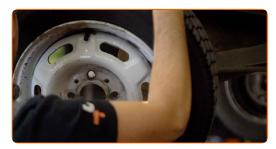
Clean the brake drum. Use a wire brush. Use WD-40 spray.
