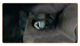
Unscrew the engine mount from the bracket. Use a drive socket #16. Use a ratchet wrench.
