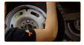
Clean the brake drum. Use a wire brush. Use WD-40 spray.
