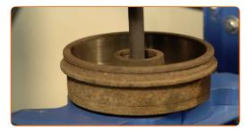
Clean the hub bearing mounting seat. Use WD-40 spray.
