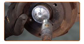
Treat the surface where the wheel rim contacts the brake drum. Use copper grease.
