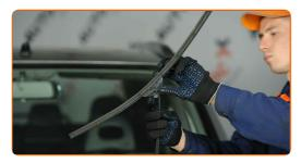
Remove the blade from the wiper arm.
