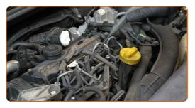
Detach the glow plug wiring connectors.
