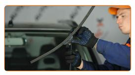
Remove the blade from the wiper arm.
