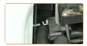
6 Connect the lock rod to the new exterior door handle and secure it with the clip.
