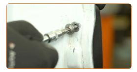
Screw in the fasteners of the exterior door handle. Use a T30 Torx bit. Use a ratchet screwdriver.
