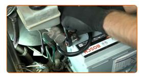
Connect the negative terminal to the battery.
