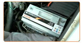
Connect the positive terminal to the battery.
