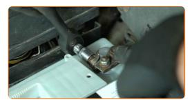
Treat the terminals with battery terminal grease.
