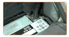
Screw in the negative battery terminal fastener. Use a 10 mm socket. Use a ratchet wrench.
