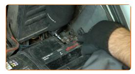
Remove the negative terminal from the battery.
