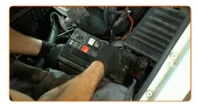
Clean the battery terminals. Use a battery terminal brush.
