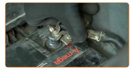
Unscrew the positive battery terminal fastener. Use an 8 mm socket. Use a ratchet wrench.
