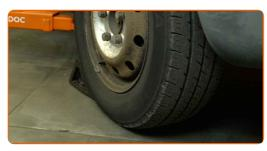
Loosen the wheel fasteners. Use a 24 mm wheel impact socket. Use a tommy bar.
