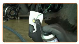
Attach the connector to the new windscreen washer pump.
