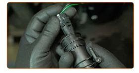
13 Install a new washer pump seal.
