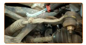
Unscrew the nut connecting the tie rod end to the steering knuckle. Use a 22 mm socket. Use a ratchet wrench.
