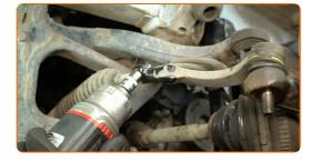
Measure and note down the length of the exposed portion of the tie rod thread or the number of turns the tie rod end made when being unscrewed to prevent wheel misalignment during reassembly. Use a vernier caliper.
