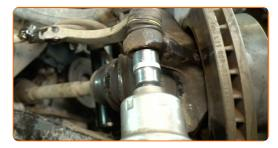
Loosen the bolt connecting the tie rod end to the tie rod. Use an 13 mm socket. Use a ratchet wrench.
