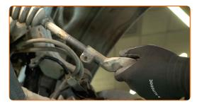
Clean the mounting seats of the tie rod end. Use a wire brush. Use an all-purpose cleaning spray.
