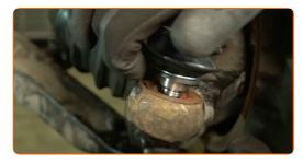
Tighten the bolt connecting the tie rod end to the tie rod. Use an 13 mm socket. Use a torque wrench. Tightening torque: 53 N·m.
