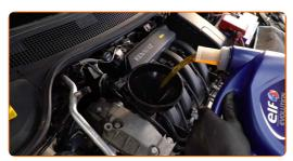
Replacement: engine oil and filter – RENAULT Master II Platform/Chassis. Tip:
