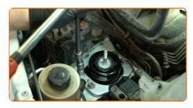
17 Install the engine mount bracket.
