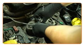
Support the engine in the area of the oil pan. Use a jack.
