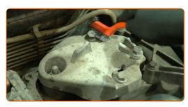
Unscrew the engine mount bracket fasteners. Use a 16 mm socket. Use a U-joint socket extension. Use a ratchet wrench.
