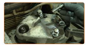
Remove the engine mount bracket.
