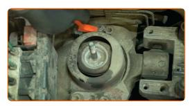
Unscrew the engine mount fasteners from the car body. Use an 18 mm socket. Use a U-joint socket extension. Use a ratchet wrench.
