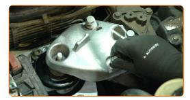
Screw in and tighten the engine mount bracket fasteners. Use a 16 mm socket. Use a U-joint socket extension. Use a torque wrench. Tightening torque: 44 N·m.
