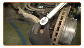
Clean the wheel rim mounting seat. Use a wire brush. Use an all-purpose cleaning spray.
