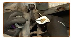
13 Attach the connector of the new ABS sensor.
