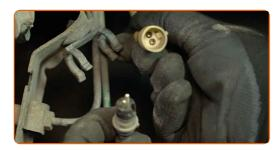
Treat the ABS sensor connector. Use an electronic spray.
