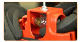
Attach the connector to the new third brake light.
