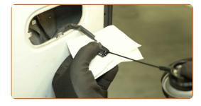
Install the bulb in the new third brake light.
