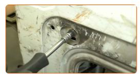
Reinstall the rear door trim cover. Use a ratchet screwdriver.
