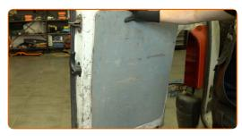
Unscrew the fastener of the third brake light. Use an 8 mm socket. Use a ratchet screwdriver.
