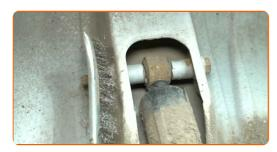
Prop up the rear axle beam. Use a transmission jack or one more vehicle jack.
