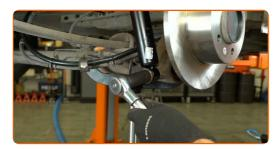
Screw in and tighten the top fastener of the shock absorber. Use a 19 mm combination spanner. Use an 18 mm socket. Use a ratchet wrench. Use a torque wrench. Tightening torque: 80 N·m.
