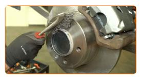
Treat the brake disc surface that contacts the wheel rim. Use ceramic grease.
