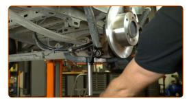
Unscrew the lower fastener of the shock absorber. Use a 21 mm socket. Use a ratchet wrench.
