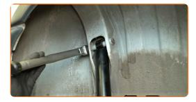
Remove the support from under the axle beam.
