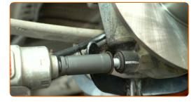
Unscrew the upper fastener of the shock absorber. Use a 19 mm combination spanner. Use an 18 mm socket. Use a ratchet wrench.
