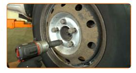
Lower the car and tighten the wheel fasteners in a criss-cross pattern. Use a 24 mm wheel impact socket. Use a torque wrench. Tightening torque: 172 N·m.
