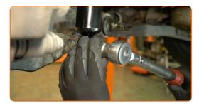
Tighten the fastener connecting the control arm to the subframe. Use a 30 mm socket. Use a torque wrench. Tightening torque: 280 N·m.
