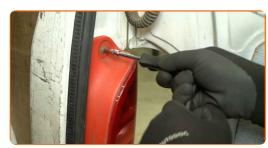
Remove the fastening bolt.
