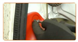
Tighten the fastener connecting the rear light to the car body. Use a T30 Torx bit. Use a ratchet screwdriver.
