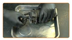
10 Remove the fuel filter cap.
