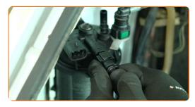
Treat the electrical connector of the fuel filter. Use an electronic spray.
