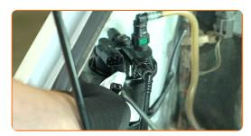
Attach the electrical connector to the fuel filter.
