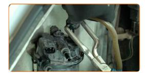
Remove the fuel filter housing.
