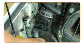
Unscrew the fuel filter cap fastener. Use a T30 Torx bit. Use a ratchet wrench.
