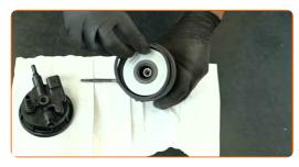
16 Install the fuel filter cap.
