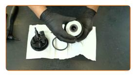
15 Install a new sealing ring.
