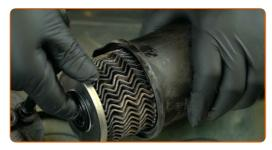
Clean the fuel filter housing, cap, and cap fastener. Use an all-purpose cleaning spray.
