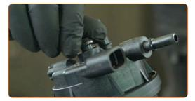
Tighten the fuel filter cap fastener. Use a T30 Torx bit. Use a torque wrench. Tightening torque: 12 N·m.
