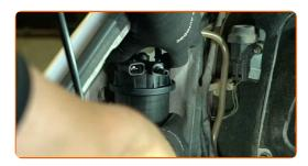
Remove the plugs from the fuel lines and connect the lines to the fuel filter.
