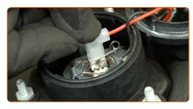
Install the fog light rear cover by turning it clockwise.
