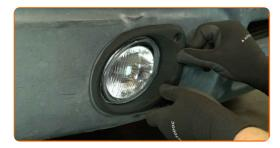
22 Install the fasteners.
