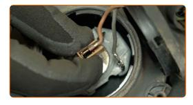
Pull aside the fog light bulb retainer.
