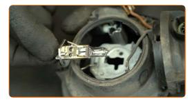
12 Install the bulb into the new fog light.
