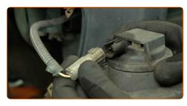
Unscrew the fog light housing fasteners. Use a T30 Torx bit. Use a ratchet screwdriver.
