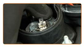
14 Attach the fog light bulb connector.
