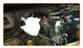
Connect the hoses to the expansion tank. Use hose clamp pliers.
