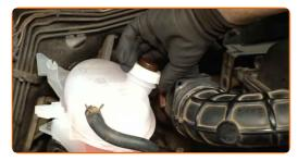
Run the engine for a few minutes. This should be done in order to remove residual air from the cooling system and to check that the components are operating correctly and there are no leaks.
