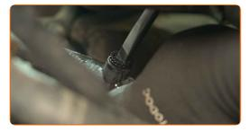
Clean the screw and the area around it to remove any coolant. Use an all-purpose cleaning spray.
