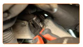
7 Unscrew the coolant expansion tank cap.
