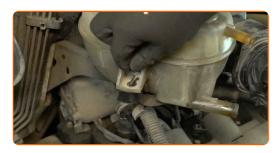
Remove the coolant expansion tank, releasing it from its bracket.
