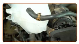
Remove the coolant reservoir cap.
