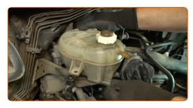
Install the new coolant expansion tank on its bracket until it clicks on.
