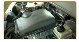
Snap the air filter cover clips into place.
