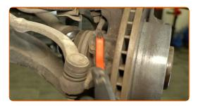
Unscrew the ABS sensor fastener. Use a 10 mm socket. Use a ratchet wrench.
