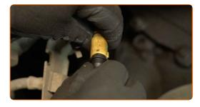
14 Secure the ABS sensor wiring.
