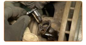
Detach the ABS sensor wiring.
