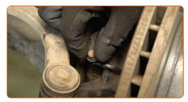
Tighten the ABS sensor fastener. Use a 10 mm socket. Use a torque wrench. Tightening torque: 11 N·m.
