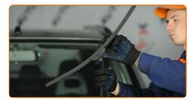
Remove the blade from the wiper arm.
