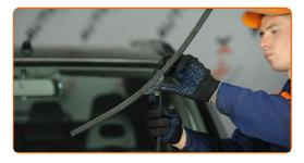
Remove the blade from the wiper arm.
