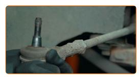
Disconnect the ball joint from the control arm. Use a combination spanner #18. Use a drive socket #18. Use a ratchet wrench.
