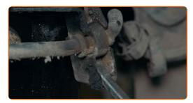
Clean the brake disc fasteners. Use a wire brush. Use WD-40 spray.
