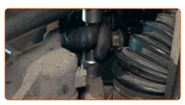
68 Connect the brake hose fastener to the suspension strut.
