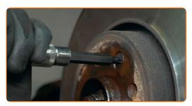
15 Remove the brake disc.
