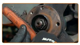
Treat the contacting surface. Use copper grease.
