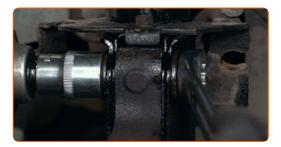
Unscrew the end fastening nut to the steering knuckle. Use a drive socket #16. Use a tap wrench.
