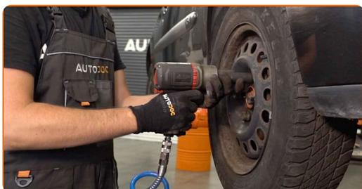
**32** Lower the car and working in a cross order, tighten the wheel bolts. Use a torque wrench. Tighten it to 90 Nm torque.
