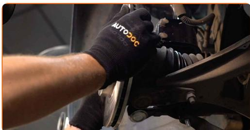
20 Tighten the brake disc fastening. Use Torx T40. Use a torque wrench. Tighten it to 15 Nm torque.
