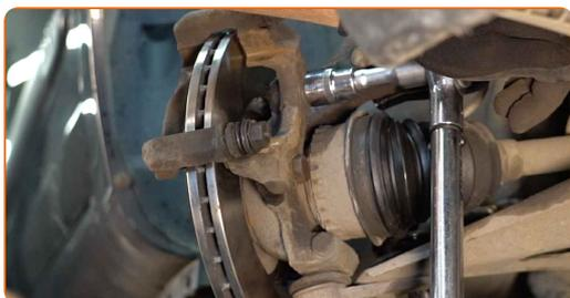
**24** Treat the brake caliper piston. Use a brake cleaner.
