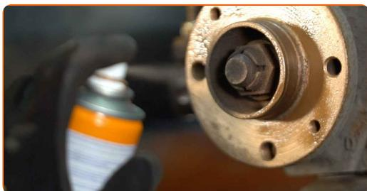
19 Install the brake disc.
