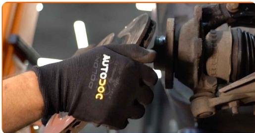
18 Clean the hub. Use a wire brush. Treat the contacting surface. Use copper grease.
