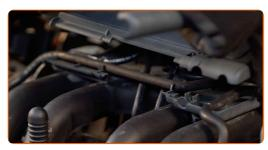
Remove the spark plug wire connectors from the spark plug wells. Use round-nose pliers.
