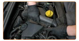
Fasten the clamp on the air intake hose. Use combination pliers.
