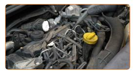
Detach the glow plug wiring connectors.
