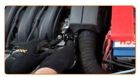
Disconnect the air intake pipe from the air filter box.
