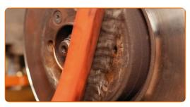
Unscrew the brake disc fastening. Use Torx T40. Use a ratchet wrench.
