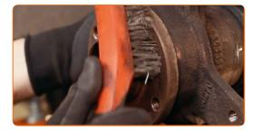
Treat the contacting surface. Use copper grease.
