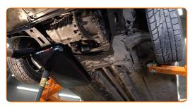
6 Unscrew the drain plug. Use square oil drain plug socket No.8
