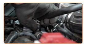
Tighten the clamp and fasteners on the air filter intake pipe. Use a drive socket #10. Use a ratchet wrench.
