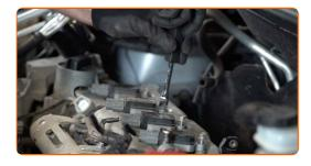
Remove the microfibre towel from the intake manifold.
